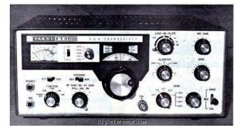
The FT-200 was advertised as a "superb quality, low cost, versatile transceiver". It covered the 80,40,20,15 and 10 meter bands with 500KHz tuning range on each band with a crystal supplied for 28.5-29MHz.
