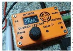
It can be used to make QRP SSB contacts, or (in combination with a PC) used for the digital modes such as FT8, JS8, FT4.
