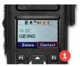
To manually dial a talkgroup on the FreeDMR or Phoenix DMR networks. First select your radio's pre-programmed (TG9 Local/Slot 1 channel) for GB3ND. On Motorola type radios press P2 or on Anytone and variants press the red button below the screen <LIST> (twice)
