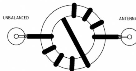
One way to **prevent common mode currents flowing in the shack**, is to insert a **1:1 Line Isolator** in the coax cable at least a quarter of a wavelength from the Unun to still allow the coax braid between the isolator and the Unun to couple to ground. The length should be for the lowest frequency band used eg 10m for the 40m band.
