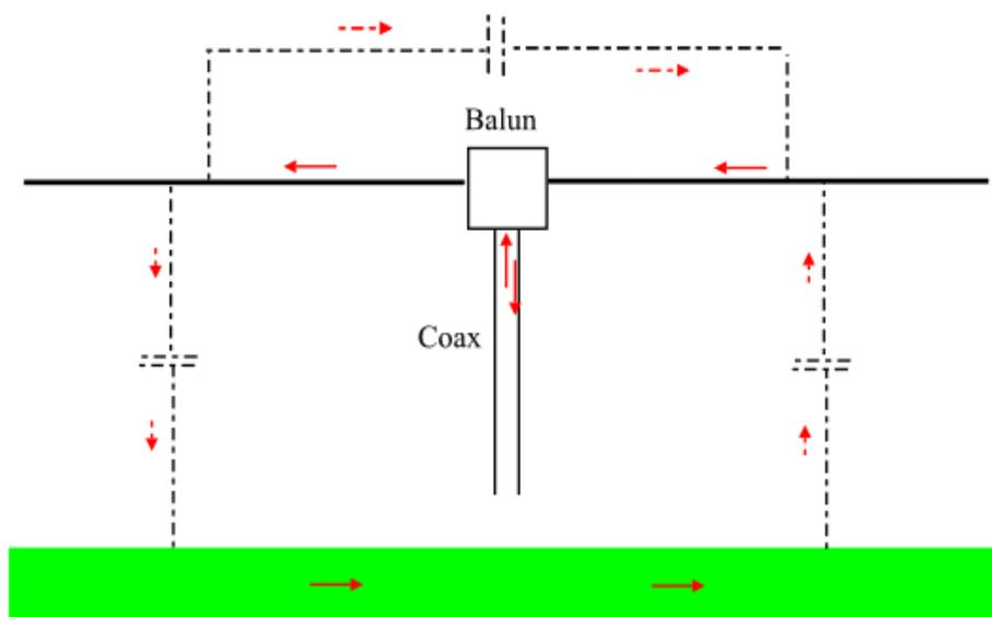
The current flows from the transceiver via the central wire of the coax and into the left arm of the dipole and the return current from the right arm flows back to the transceiver via the inner surface of the coax outer. But how is the circuit completed? Two possibilities are shown in the above diagram :-
