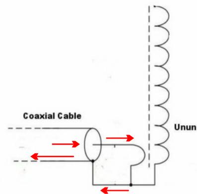
Now connect the end fed antenna wire to the Unun :- (Note there is no direct earth connection between the Unun Ground terminal and earth)
