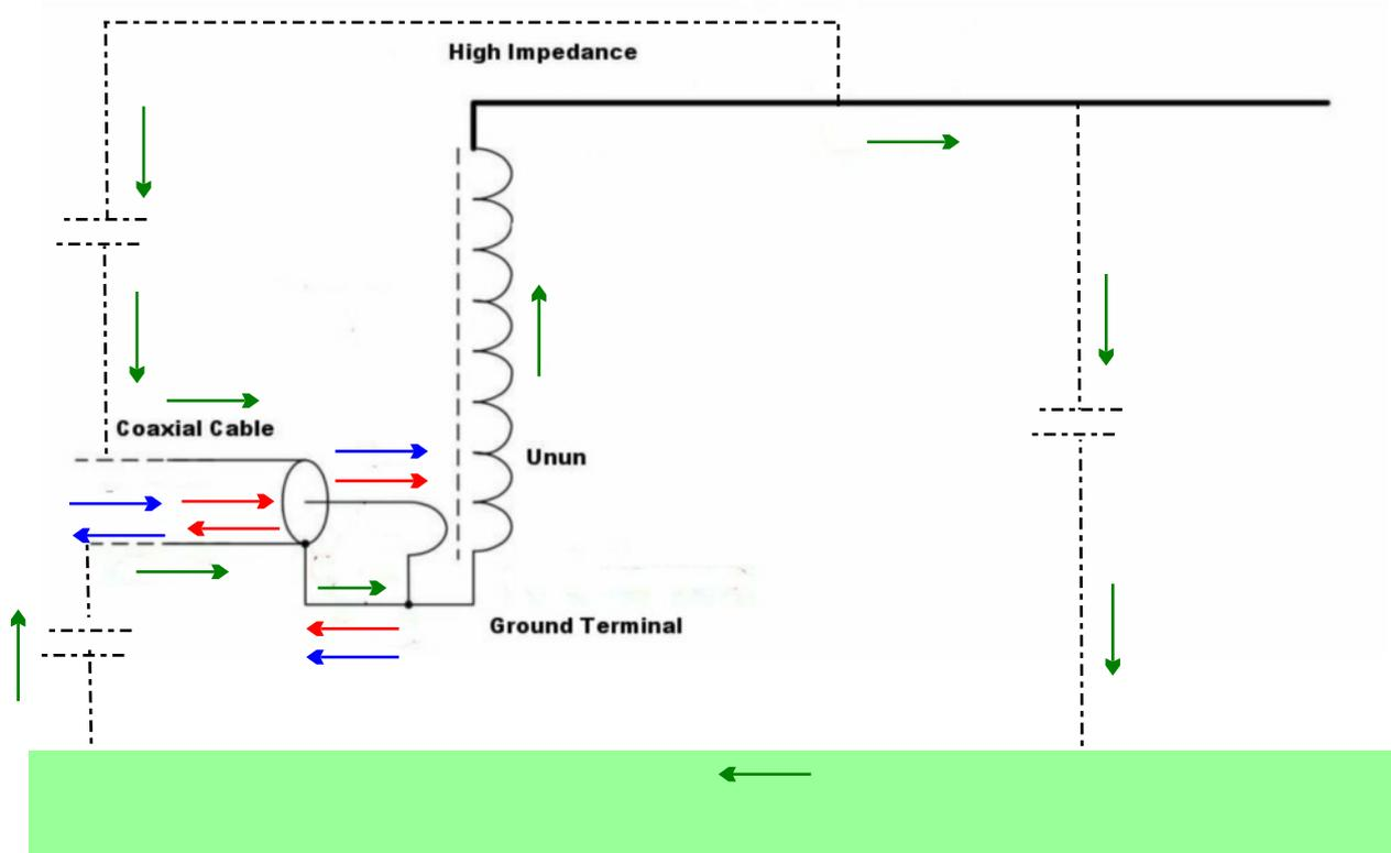
Assuming that the analysis of current flow in a dipole is correct ie the current circuit is completed via either direct capacitive coupling or via the ground then as shown in the diagram above, there appear to be two possible ways in which the circuit is completed - namely by direct capacitive coupling between the antenna and the coax outer, or via capacitive coupling with the ground.
