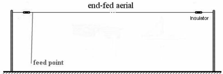
Consequently the feed point can be either elevated or near ground level. Also the antenna length can be a resonant length (ie multiple of half wavelengths) or non resonant which will influence what bands the antenna can operate on.
