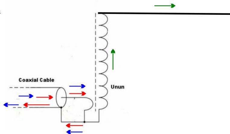
However, the current in the antenna wire will only flow **if there is a complete circuit** which begs the question as to how the circuit is completed.
