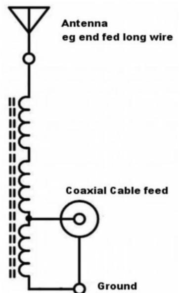
Commonly used impedance ratios are 9:1, 49:1 and 64:1. As will be explained later, 9:1 Ununs are used with non resonant multiband end fed antennas, whereas resonant end fed antennas with their much higher end impedance require a 49:1 or 64:1 Unun.
