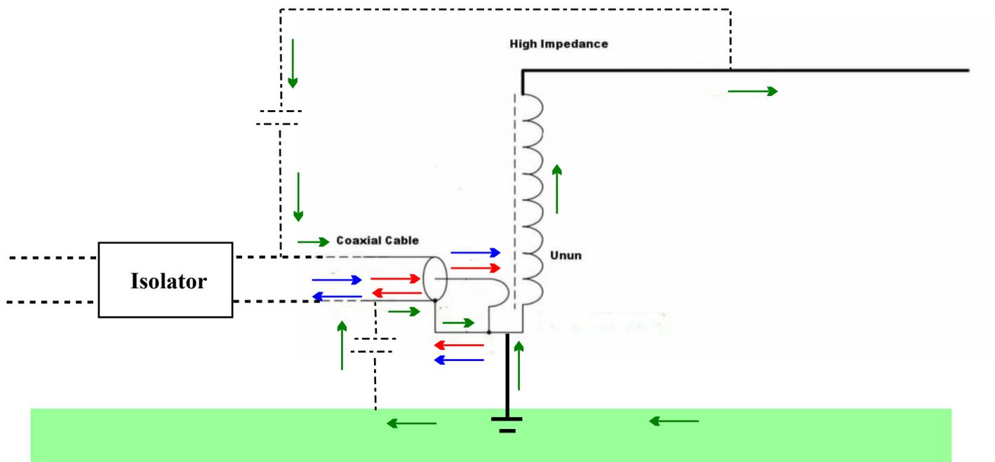
The earthing wire from the Unun Ground terminal to the Earth rod should be as short as possible and definitely much shorter than a quarter of a wavelength at the lowest frequency in use. This may prove difficult for an antenna system using an elevated feed.
