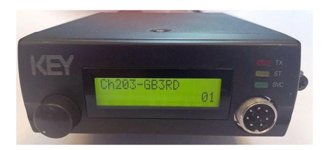
These VHF radios are preprogrammed for 2m frequencies. The radio supports a maximum of 256 channels and these include all the simplex channels as well as all the current (at time of programming) 2m analogue repeaters. As supplied CTCSS is programmed for both receive and transmit so annoying digital signals will not open the squelch if the repeater is dual mode FM and digital. You can change these options with the free, downloadable, programming software.
