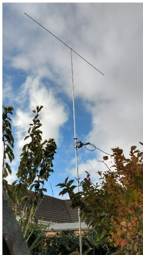
As can be seen from the above photo, the antenna is not in the best position, the lower horizontal capacity hat being only just over a metre away from and parallel to the return coax to the shack!
