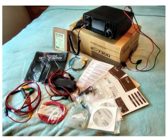
As can be seen it comes with the RT Systems programming lead, two spare DC leads, the Sotabeams Click2Tune adaptor, unused matching Icom cover, fuses etc ..
